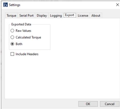
The export tab sets up the parameters for the Excel .csv file. It allows you to choose whether you want to export the Raw Values from the RX10K, the Calculated Torque from the shaft parameters, or both. You also have the choice to have column headers appended to the data.
