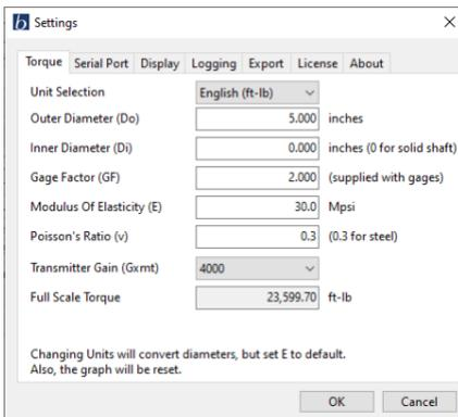
The Torque tab is used to configure the shaft properties and gain setting. The default units are English ft-lb, but English in-lb, and Metric units can be selected from the drop-down Unit Selection menu at the top.
