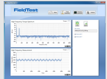
High frequency acquisition screen For torsional vibration analysis
