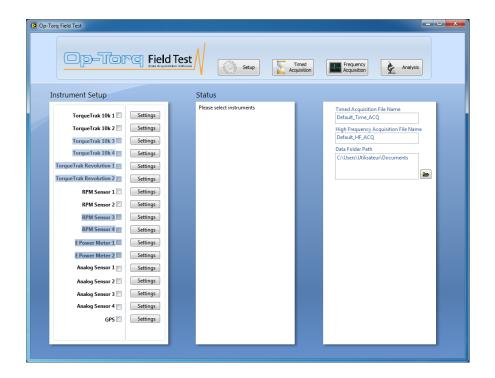
On the SETUP screen, the STATUS box shows the status of all selected instruments. This is a valuable indicator to diagnose a connection or a calibration problem.
