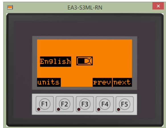
The Torque screen acts as the Home screen. Press F5(next) to cycle through the main menus. Pressing F3(scrn) provides access to submenus and screens.
