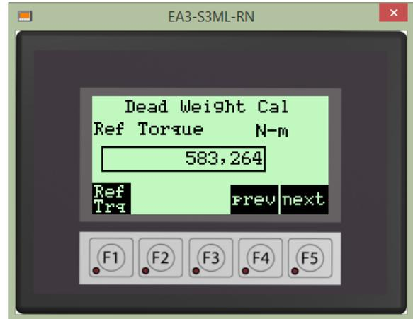
The Reference Torque capture screen works just like the Rest Torque capture screen. The only difference is that it captures the Reference Torque TPM2 value.
