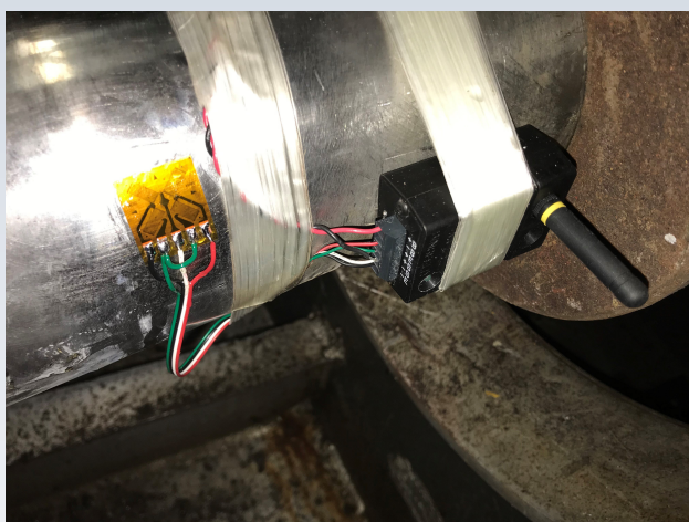
Figure 3. A portable battery-powered system (left) and a permanently installed inductive system (right).
