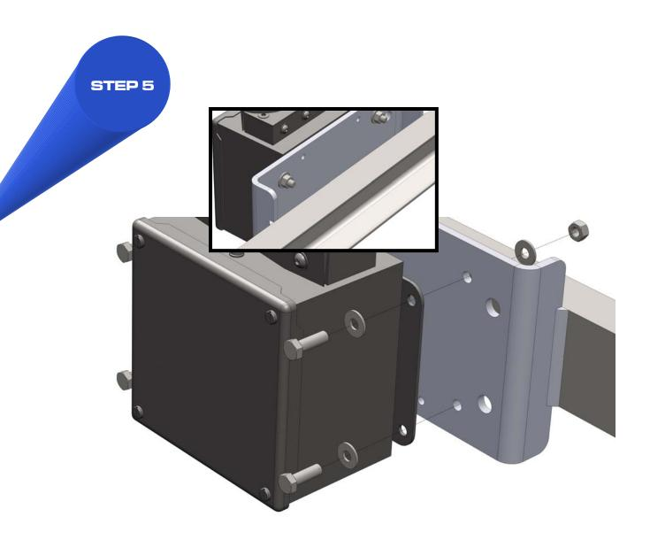
Install the Torque-Trak Revolution enclosure by using the 5/16" hardware provided with the kit.
