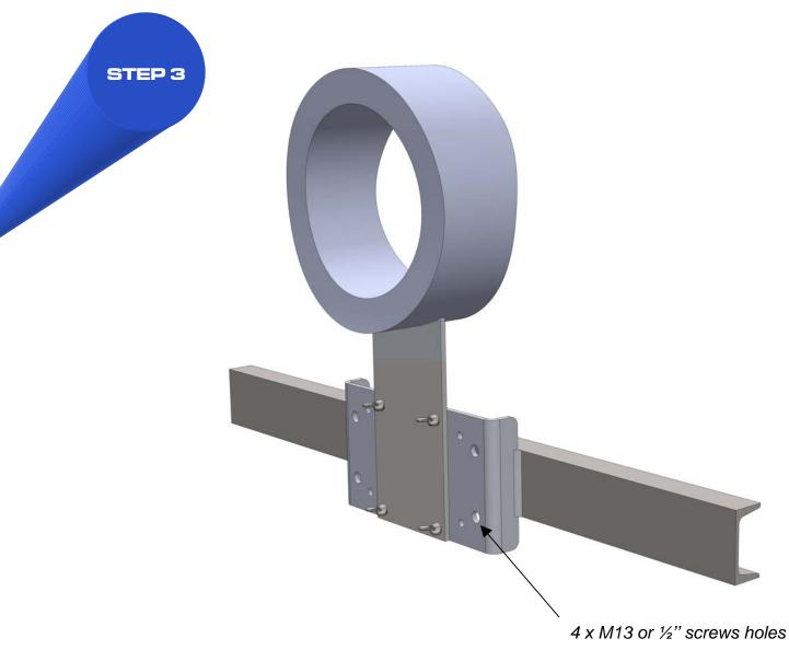
Mate the spacer with the shaft and weld the bracket on a previously installed steel beam.
