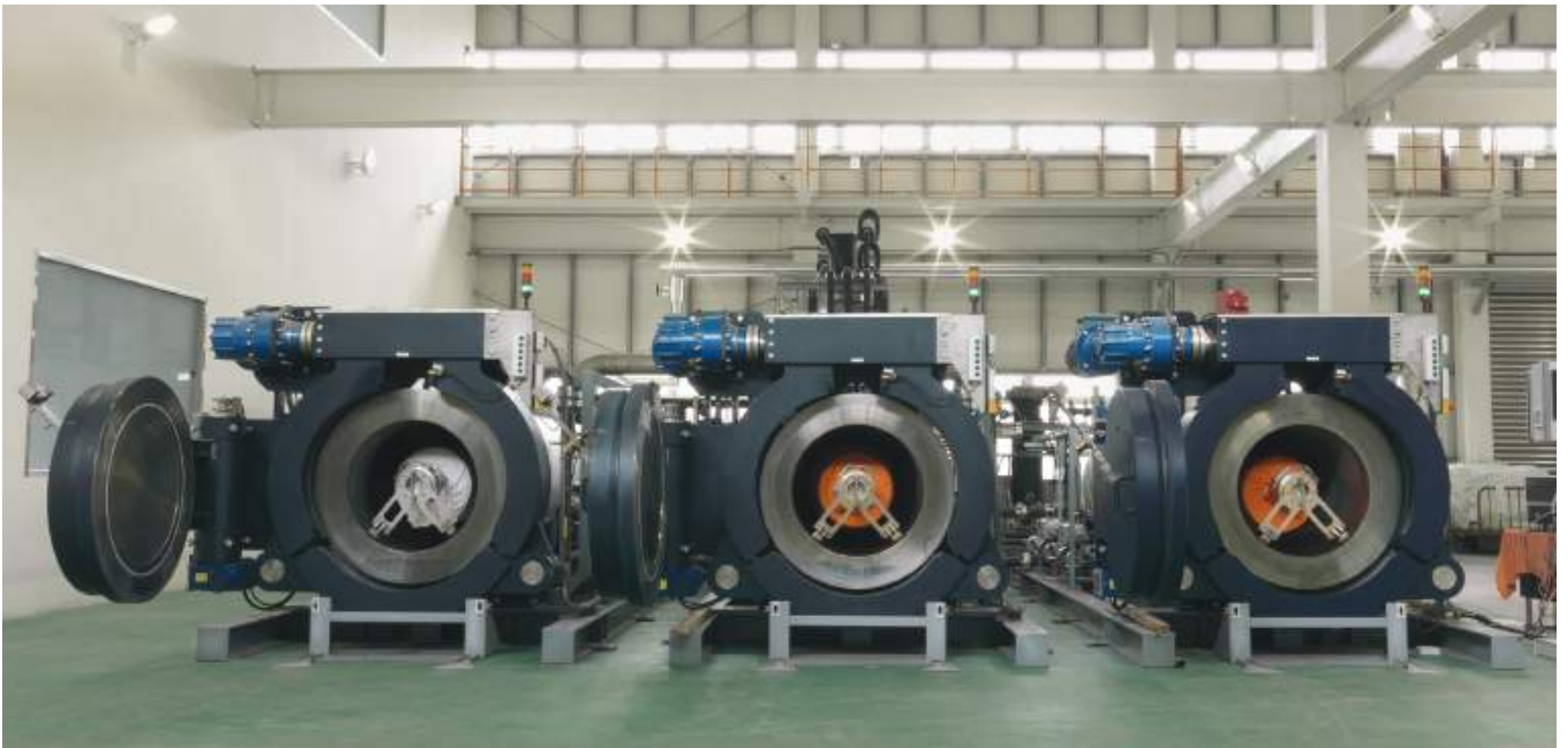
DyeCoo's technology consists of three vessels
