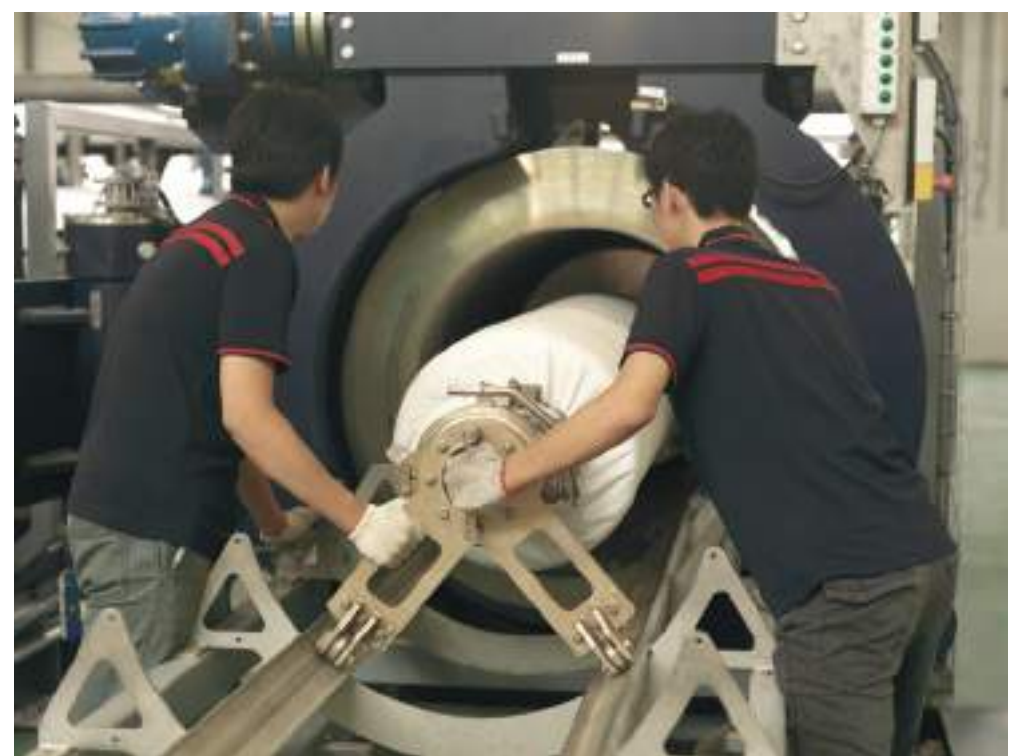
Loading fabric into the vessel
