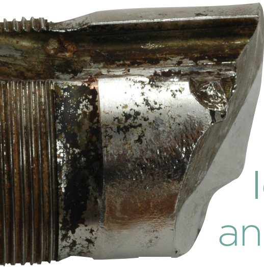
Figure 1: Torsional fatigue fracture of a pump shaft with fracture face 45 degrees to the shaft
