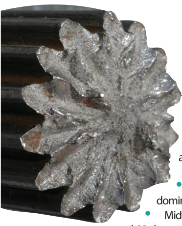
Figure 4: Reversed torsional fatigue failure of a splined shaft; each spline has two cracks, each at 45 degrees to the shaft
