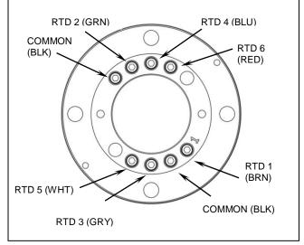
Rotor-RTD Wiring Diagram (Note color code)
