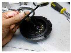
Fig. 6 - Stator Top Plate with Gland
