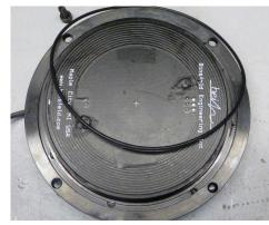
Fig. 3 - Stator Plate with Electronics
