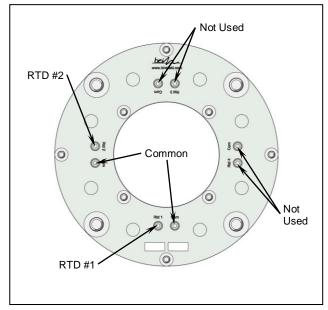
Rotor/RTD Connections Diagram
