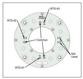
Rotor/RTD Wiring Diagram
