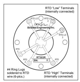
Rotor/RTD connections Diagram
