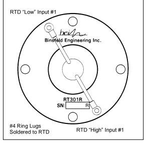
Rotor/RTD Connection Diagram
