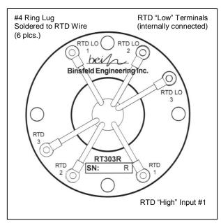
Rotor/RTD Wiring Diagram
