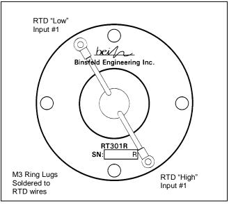
Rotor/RTD Connections Diagram
