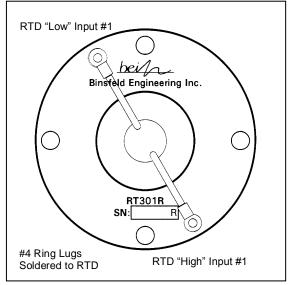
Rotor/RTD Connection Diagram
