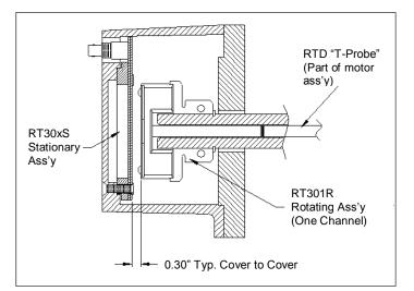
Complete System Assembly Diagram
