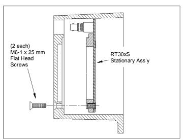
Stationary Assembly Installation Diagram
