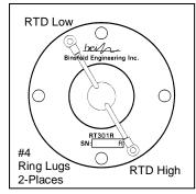
Rotor/RTD Connection Diagram
