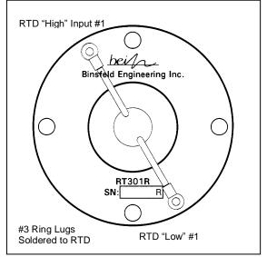
Rotor/RTD Connection Diagram
