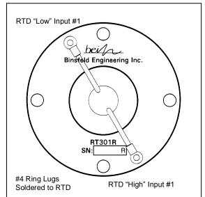
Rotor/RTD Connection Diagram
