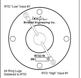
Rotor/RTD Connection Diagram
