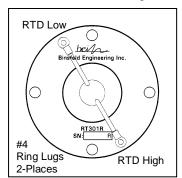
Rotor/RTD Connection Diagram
