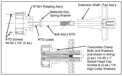
Bolt & Rotary Ass'y Installation Diagram
