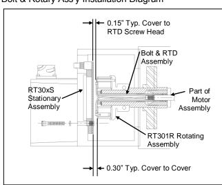
Completed RT301 Installation Diagram
