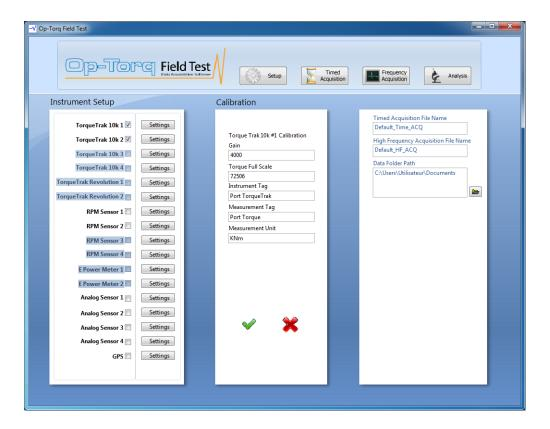
On the right side of the screen, enter the target name and folder where you want to save acquisition files on your computer. The file names are incremented as to prevent overwriting.
